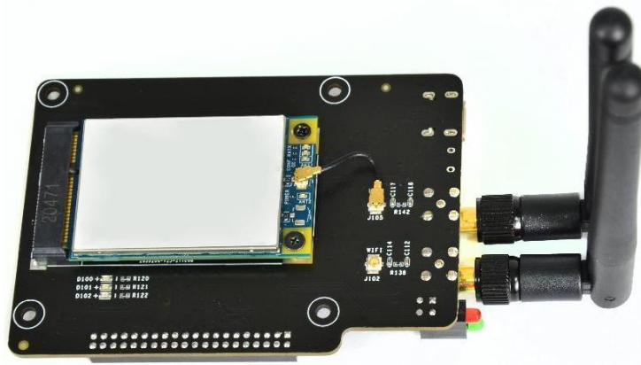
Figure 9 Connect DEBIX LoRa with antenna
