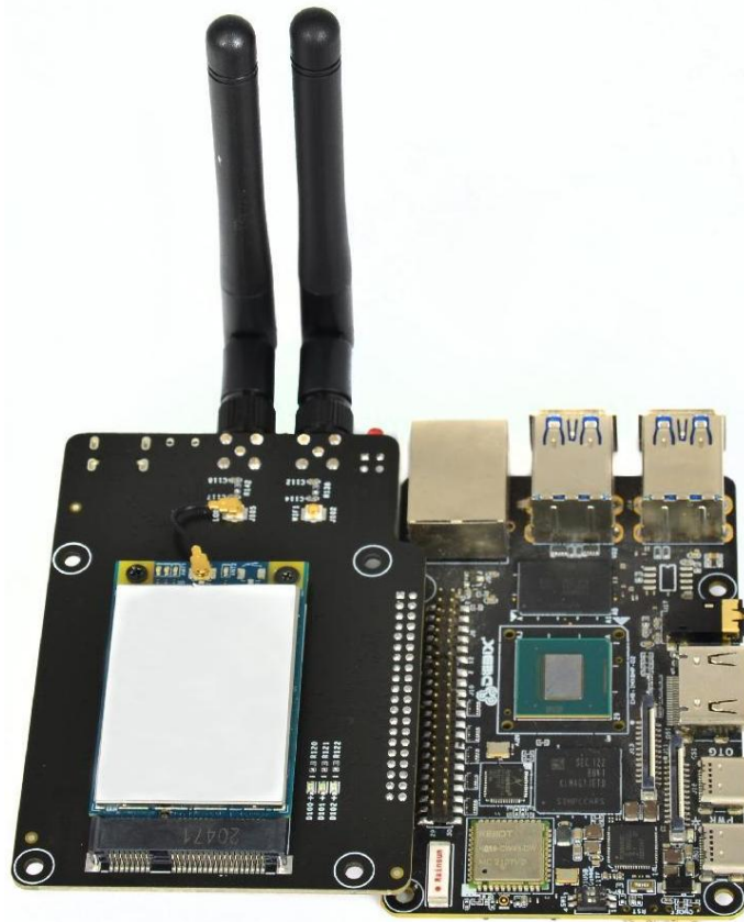
Figure 12 Connect DEBIX with DEBIX LoRa board
